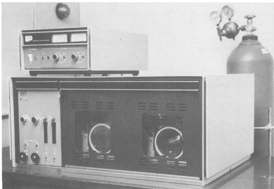
FIG. 1—Instrument used for oxygen plasma ashing.
